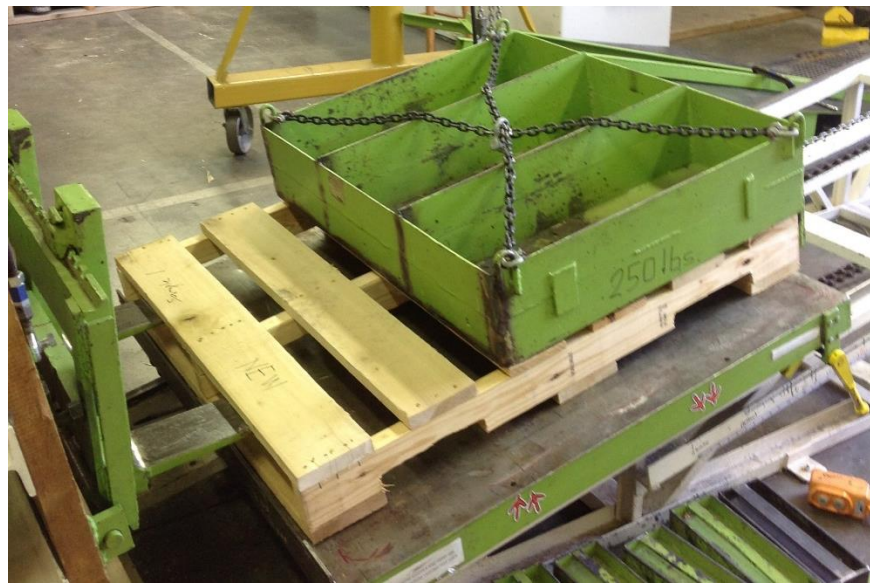
Figure 6 Experimental setup for incline impact test on pallet edges.
