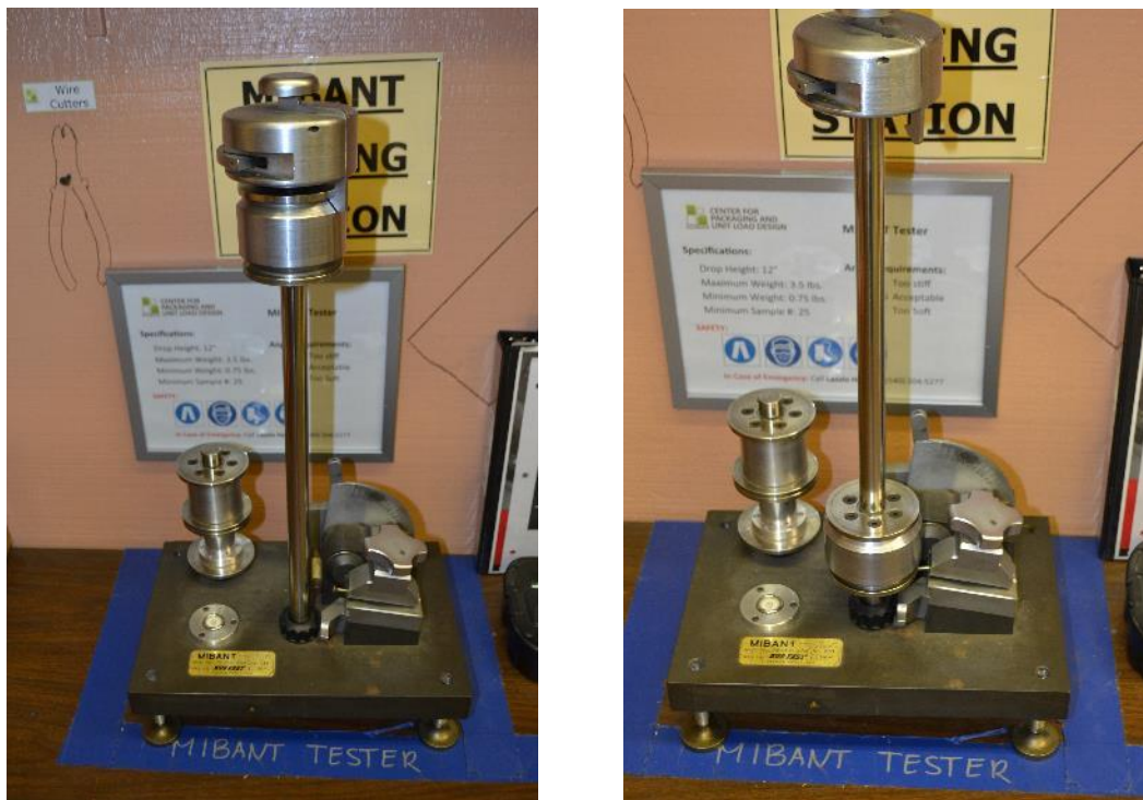
Figure 4 Experimental setup for the MIBANT test.
