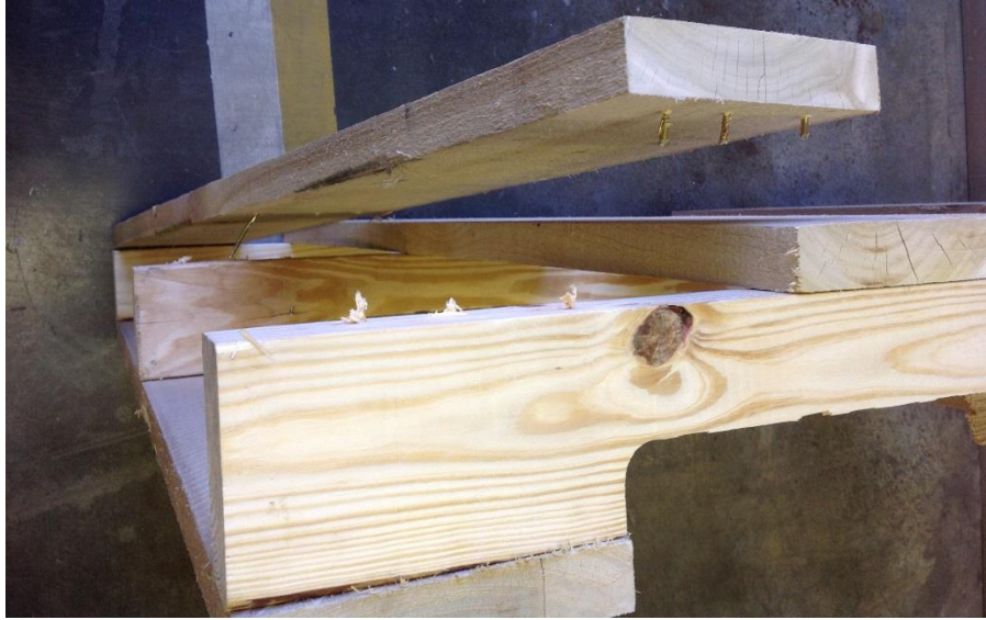
Figure 7 Representative mode of failure of the investigated pallet design during the incline impact test on pallet edges.
