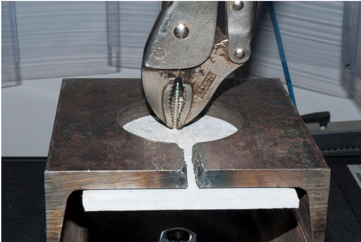
Figure 2. Typical Screw Pull Through Setup
